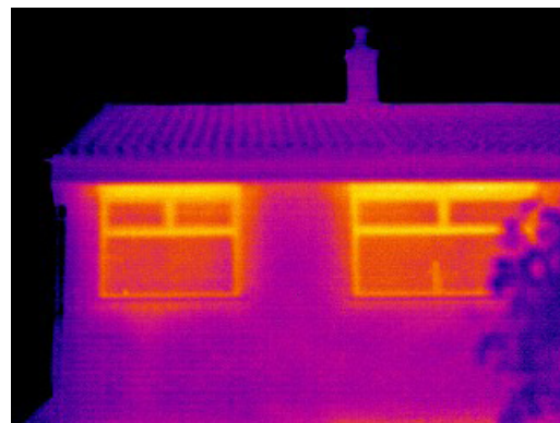
Thermal images clearly showing heat loss
